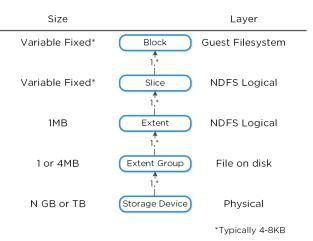
Figure 3.2-3. Low-level Filesystem Breakdown
