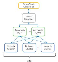
The figure shows an example of scaling OVMs for a single site:
