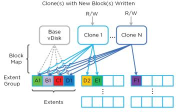
Figure 3.2-35. Clone Block Maps - New Write
