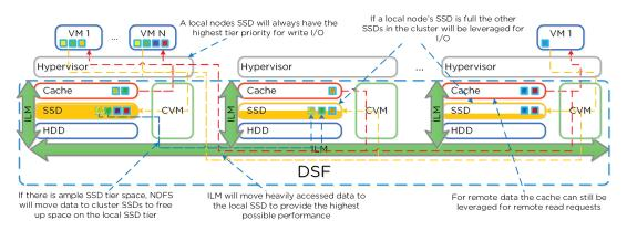
Figure 3.2-27. DSF Cluster-wide Tier Balancing
