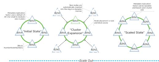
The following figure shows an example of the metadata "ring" and how it scales:
