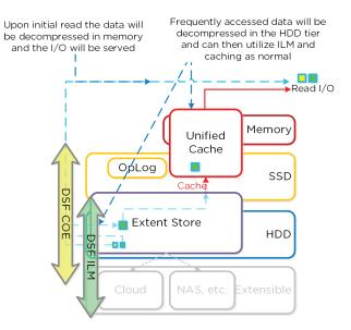
Figure 3.2-22. Decompression I/O Path
