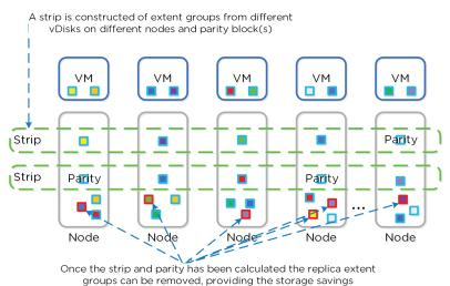
Figure 3.2-18. DSF Encoded Strip - Pre-savings
