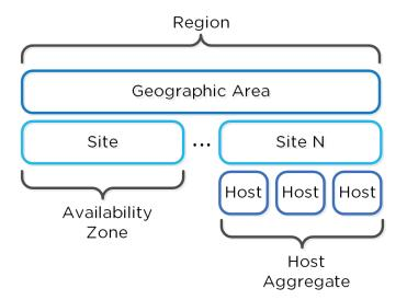
Figure 2.6-8. OpenStack - Deployment Layout
