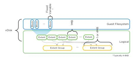
Figure 3.2-4. Graphical Filesystem Breakdown
