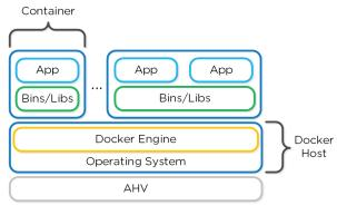
Figure 3.3.30. Docker - High-level Architecture
