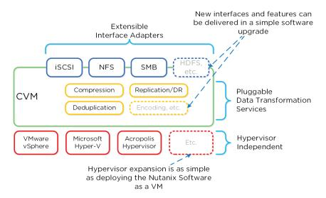
Figure 3.1-3. Software-Defined Controller Framework
