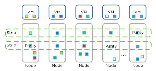
Figure 3.2-19. DSF Encoded Strip - Post-savings
