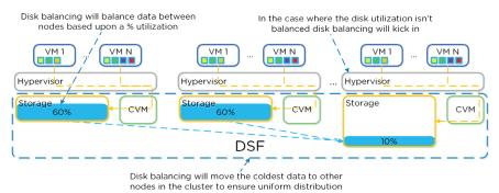
Figure 3.2-29. Disk Balancing - Unbalanced State
