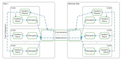
Figure 3.4.21. Replication Architecture - SSH Tunnel
