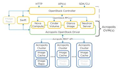
Figure 2.6-2. OpenStack + Nutanix API Communication
