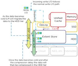
Figure 3.2-21. Offline Compression I/O Path
