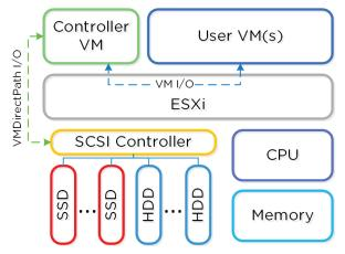
Figure 5.1.1. ESXi Node Architecture
