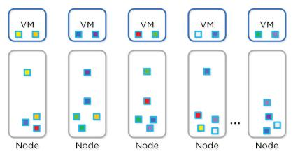
Figure 3.2-17. Typical DSF RF Data Layout
