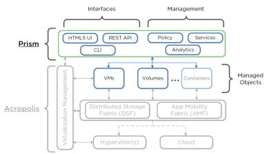
Figure 2.2-1. High-Level Prism Architecture
