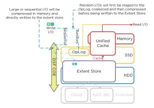
Figure 3.2-20. Inline Compression I/O Path
