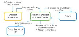
Figure 3.3.33. Docker - Container Creation Workflow You now have a container running with persistent storage!
