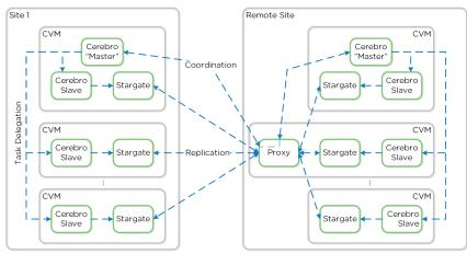
The following figure shows a representation of the replication architecture using a proxy:
