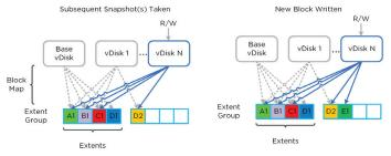
Figure 3.2-33. Multi-snap Block Map and New Write
